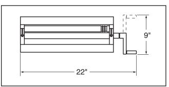
Figure 5. T21323 Minimum working clearances.
